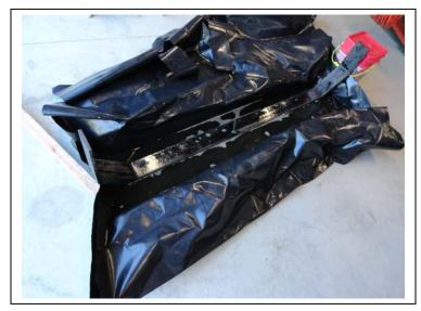
By utilizing a piece of plastic sheeting and several pieces of stray timber, a cheap and simple dip tank can be created to enable the de-rusting of larger items. By building the sides up with timber and laying the plastic sheeting inside the timber frame, a simple but effective dip tank can be created for a minimal expense. Once the de-rusting has been completed, the Evapo-Rust can be scooped out and put back into a storage receptacle for later use.
